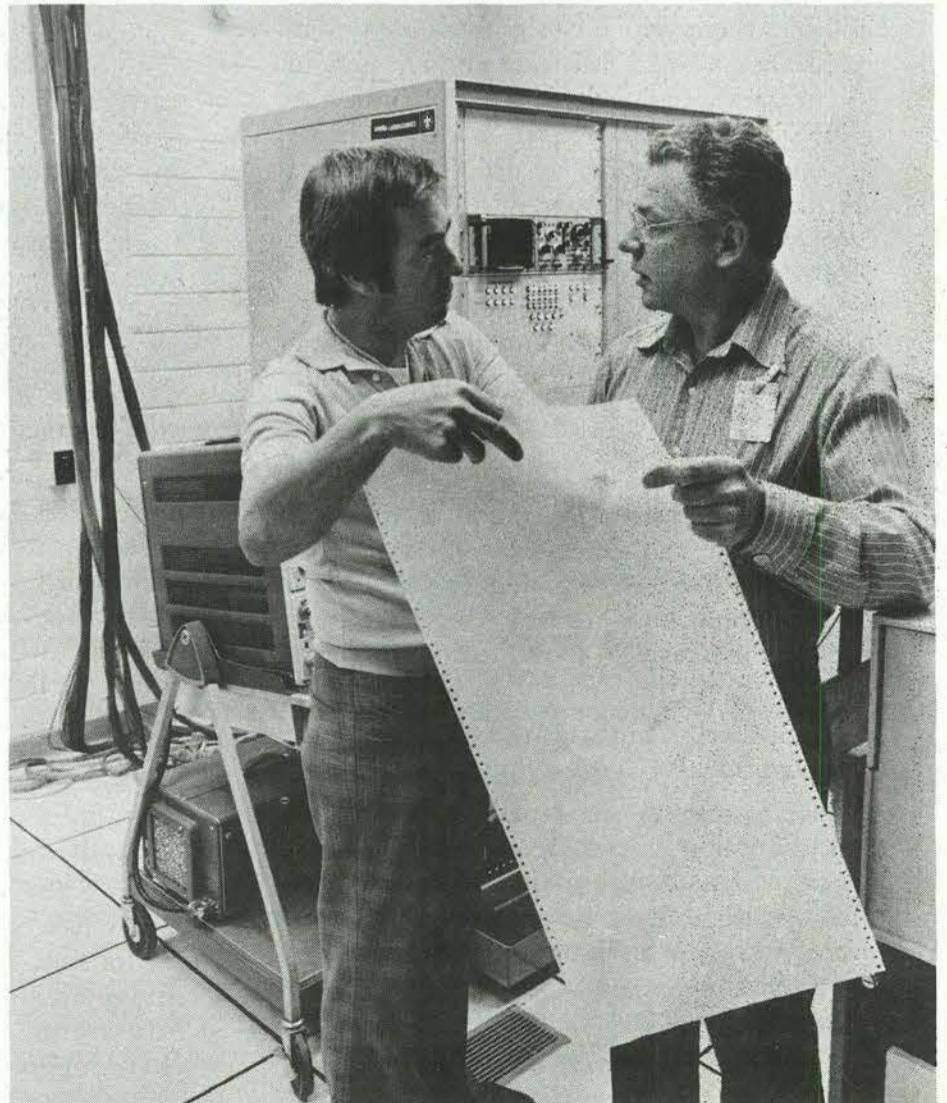
operation. Test systems are connected directly to an EMR 6135 computer which provides real-time readout. High altitude environments in excess of 300,000 metres ( 1.7 \times 10^{-5} pascals) and thermal environments from -62^{\circ}\text{C} to 50^{\circ}\text{C} are provided. Ken checks data with Don Gorsline (1242), right.
